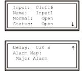
Each Main Module supports up to 16 user-defined input contacts. Each contact monitors a sensor and responds to changes in the state of the sensor (open or closed).
